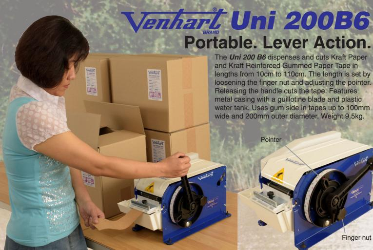
The *Uni 200 B6* dispenses and cuts Kraft Paper and Kraft Reinforced Gummed Paper Tape in lengths from 10cm to 110cm. The length is set by loosening the finger nut and adjusting the pointer. Releasing the handle cuts the tape. Features metal casing with a guillotine blade and plastic water tank. Uses gum side in tapes up to 100mm wide and 200mm outer diameter. Weight 9.5kg.
