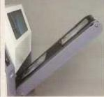
Take-away Conveyor (optional) The optional take-away conveyor can be attached in minutes. It fits the front (as illustrated) or back of the machine and has a durable rubber belt with ridges to transport the finished articles to packing bench height
