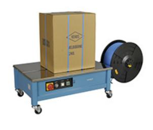
The VHPE10DL Low Tabletop Strapping Machine is built lower to the ground to allow for easy strapping and movement of tall and heavier boxes on and off the table. This semi-automatic strapping machine takes 6, 9, 12 and 15.5mm PP strapping and uses convenient single phase power. It also comes with a strap length timer to pre-set strapping length and lockable castor wheels.
