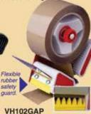
Metal and plastic with antirust blade, plastic roller and rubber guard that exposes the blade only when cutting tape. Large finger nut for easy brake adjustment. Takes rolls to 50mm wide and 120mm outer diam, on a 76mm core. Wt. 350g
