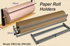
Heavy cast iron supports, steel guide bar with aluminium straight tear edge, wooden dowel spindle and timber base. The tear edge screws on and off for easy replacement. Maximum roll outer diam. 260mm (subject to weight). Available in 1140mm and 1520mm widths.
