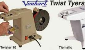
Uses 4mm wide TIEFIX Twister 10 plastic coated wire ribbon available in white, red, blue, gold and silver on 500m spools and white on 900m spools. Cuts an 85mm length and twists it around the necks of bags at up to 50 bags per minute. Suits bag neck diameters to 12mm. Dimensions with spool: 520mm x 180mm x 280mm high. Weight 7kg.
