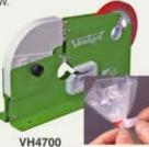
Metal construction. Uses 9mm wide PVC tape to 120mm outer diam. on a 76mm core and 9mm wide paper roll to 75mm outer diam, on a 25mm core. A single action seals the bag and applies paper to exposed adhesive surfaces. Twisted neck diam. 12mm. Wt. 1.02kg.
